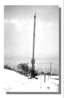
The equipment delivers an unmatched 500 ton per square foot of driving force, combining static and dynamic forces to penetrate the stiff underlying striates eliminating the need to auger or drill in most soil conditions.
